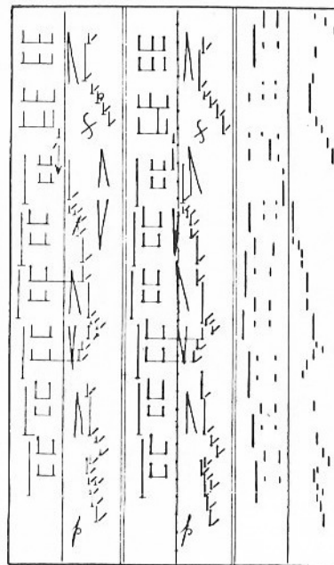
26 Making a perforated strip. Left: a passage from Chopin's Waltz op. 19 No. 1 (posthumous) recorded on the strip by a pianist. Centre: The strip after corrections have been made—ready for perforation. Right: The perforated strip is ready for reproduction.
